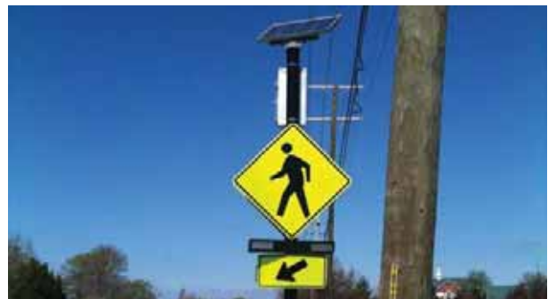
Rectangular Rapid Flashing Beacon (RRFB)
