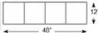
12" x 12" Slate Border FM-3300 S/O 12" x 48" (30.48 x 121.92 cm) Red A border of four 12" slate squares in a row Matching skin/touch-up wheel: Smooth Slate/TW-5 Joint size 1/2" wide, 1/2" deep
